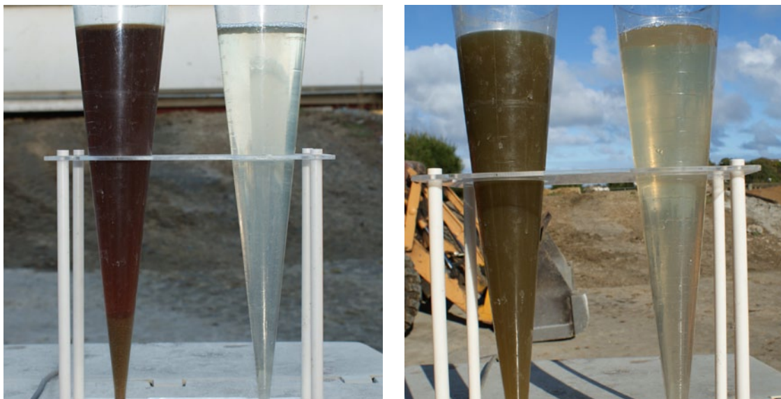
Chemically Assisted Filtration (or CAF) for separation of colloidal matter from raw effluent.
